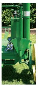
Convenient lever operated hydraulics with 2 double sets of quick couplers.
