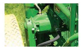
Ground driven pump and accumulator system develops live hydraulics to operate cylinders on towed equipment. New is an improved, unique system to completely unload the hydraulic pump immediately after oil is recovered.
