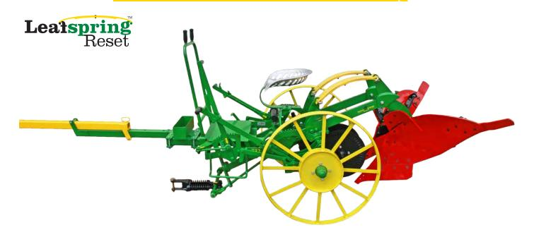
The model #732 2-way sulky plow allows for plowing the same furrow in both directions, which eliminates dead furrows in the middle of field. This capability makes the model #732 a popular choice for produce farmers that do double cropping and narrow strip farming. It is also widely known as a hillside plow where continuous uphill plowing is necessary to reduce erosion.
