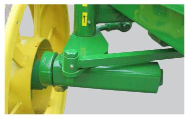
Optional torsion axle suspension provides a smooth ride and shock protection for implements and operator.
