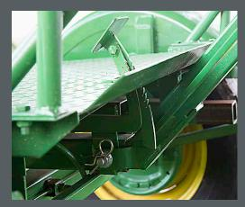
Optional heavy duty hydraulic brakes with foot pedal parking brake lock.
