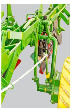
Ground driven mechanical clutch
