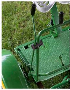
Hand crank allows axle to move forward or backward, balancing the weight over the wheels and reducing the load on the horses.
