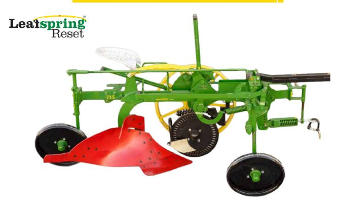
Model #715 leaf spring reset, the first sulky plow in production that automatically resets over rocks.
