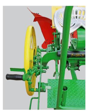
Foot activated wheel lift will fully raise bottom to a set position without using hand lever.
