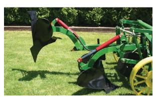
Double pivot beam allows exceptionally high clearance over rocks.
