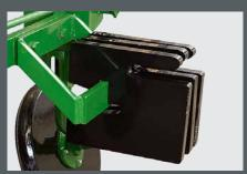
Three 35 lb. weights mounted on standard bracket
