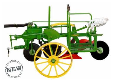
Optional bolt-on platform with front and side safety railings allows operator to stand while plowing for better visibility over horses.
