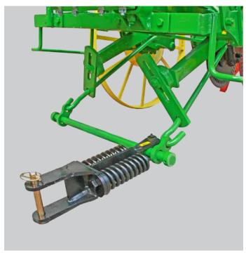
Full range draft adjustment with self-sliding spring hitch.
